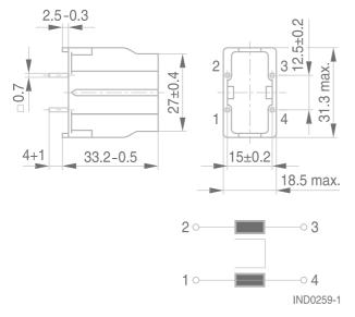
Part tolerances to ISO 2768-cL / ISO 8015. Size ISO 14405 (E) All dimensions in mm
